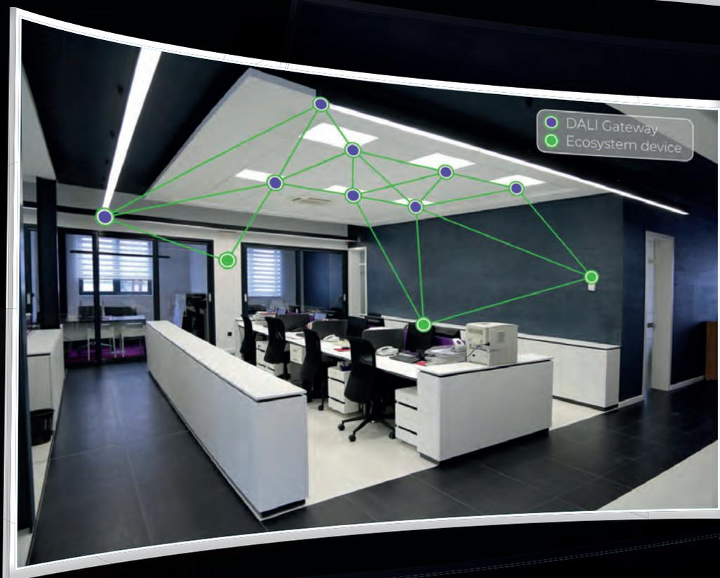
Standardized gateways allow existing DALI wired products to be used in either Bluetooth® mesh or Zigbee® wireless ecosystems. Gateways translate between protocols, and DALI control gear can report luminaire, energy and diagnostics data to the wireless network.
